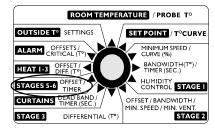
(Press the push-button four times to display the Stage 6 offset). Use the adjustment knob to set offset to the desired value.
