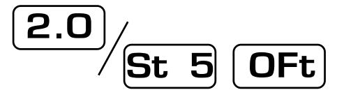
(ii) If, after about 6 seconds, no action is taken by the user, the absolute temperature value is displayed, alternating with "St 5" and "StP". In this case, the absolute value is: Set Point + Stage 5 Offset.
