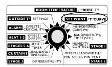
Press the push-button. The word **OFF** is displayed indicating that the termperature curve is deactivated. If this is not the case, see below to deactivate the curve.
