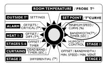
**NOTE:** The minimum speed can be adjusted only if the minimum speed curve is deactivated or if the minimum speed curve is activated but not currently operating (see below).
