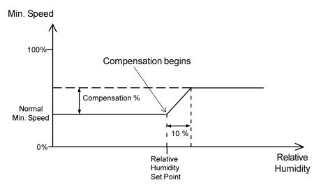
This feature also applies when the minimum ventilation speed is activated. Note that for the compensation to take place, the compensation feature must be activated by the user. When a compensation is applied to the minimum speed, the compensation pilot light turns on.
