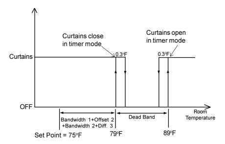
In the example above, when the temperature rises to 89°F, the curtains begin to open and continue to do so until fully open if the temperature remains above this point. If the temperature falls to 88.7°F, the curtains stop opening. When the temperature falls to 79°F, the curtains begin to close and continue to do so until fully closed if the temperature remains below this point. If the temperature rises to 79.3°F, the curtains stop closing.
